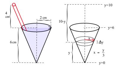
In this example, both the force and the distance vary, and each depends on the height of the "slice" above the bottom of the cone.
