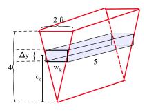
We integrate from y = 0 to y = 4 because the bottom slice of liquid is at a height of 0 feet and the top slice of liquid is at a height of 4 feet.
