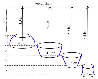
The work needed to move each slice is approximately the weight of the slice times the distance the slice is moved. We can use the radius at the bottom of each slice to approximate the volume — and then the weight — of the slice, and a point halfway up each slice to calculate the distance the slice is moved. For the top slice:
