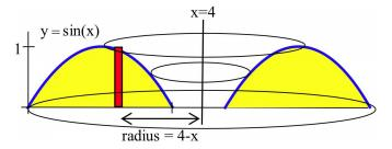
Vertical slices again generate tubes when rotated about x = 4; the only difference here is that the radius for a slice located x units away from y-axis is now 4 - x (the distance from the axis of rotation to the slice). The volume integral becomes:
