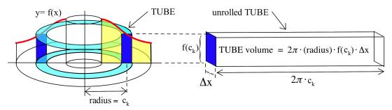
to get a thin, solid rectangular box. The volume of the tube is approximately the same as the volume of the solid box:
